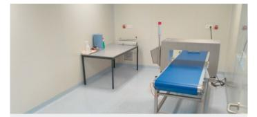
Cleanroom with a metal detector for detection of ferro, non-ferro and stainless steel contamination in packaged powders (450 mm width x 250 mm height).
